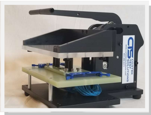
Flip Top Mechanical Press for testing fine pitch contacts PCB.
